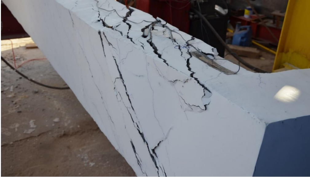
Figure (8) Specimen T2 after failure
