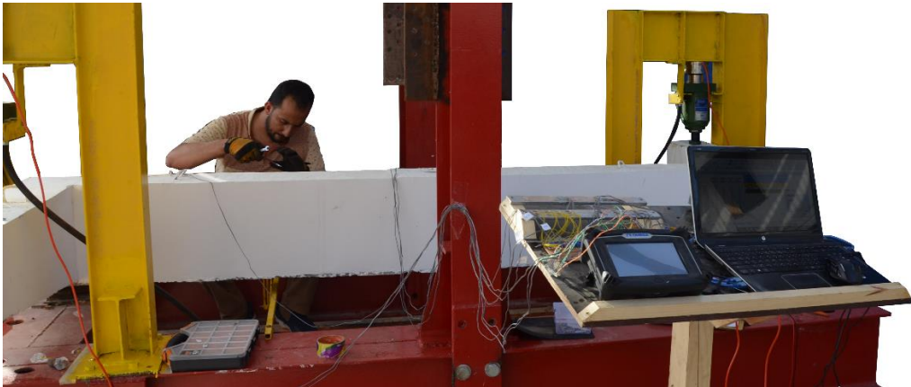
Figure (6) Setup for the torsion test (Testing rig, strain gauge data logger, and load cell data logger)
