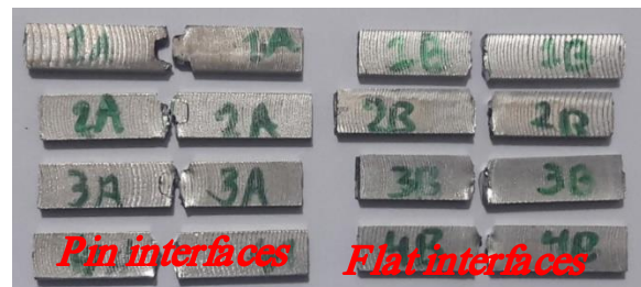
Figure 8 Specimens after completion of impact tests
