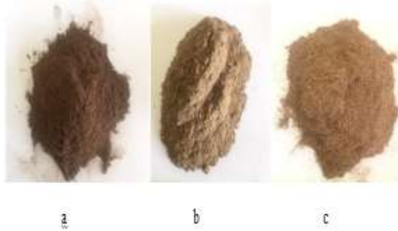
Figure 1. samples of palm fibers: (a) Sample with diameter 75µm (b) Sample with diameter 125µm (c) Sample with diameter 140µm.
