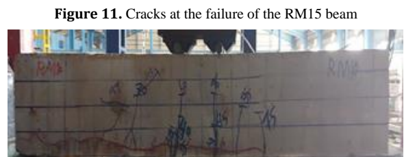
Figure 11. Cracks at the failure of the RM15 beam
