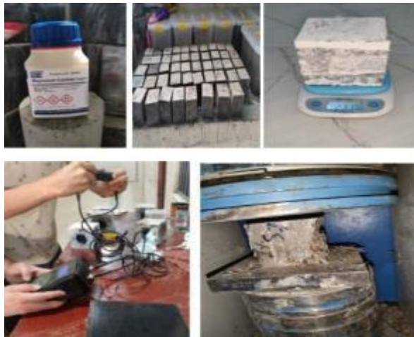
Figure 4 Sulfate Impact on SCC Test
