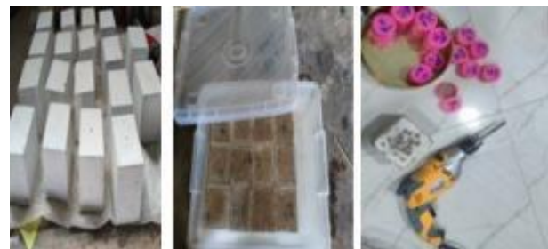
Figure 5 Chloride Penetration Test Process.
