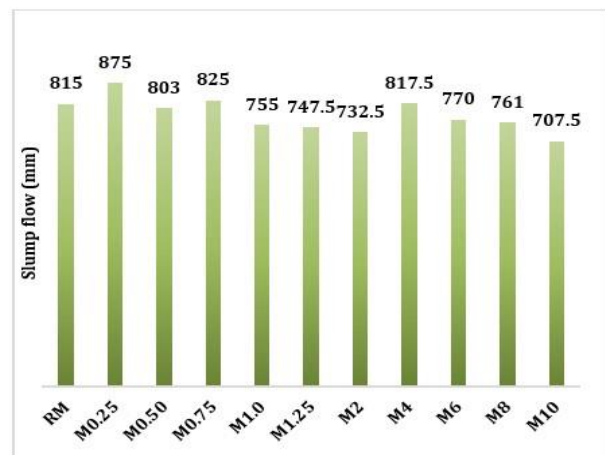
Figure 6 Slump Flow Diameters for SCC Mixtures
