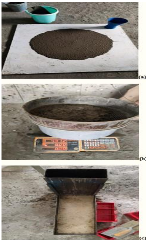
Figure 2 Fresh properties tests (a) Slump flow resistance (b) Segregation (c) Blocking ratio
