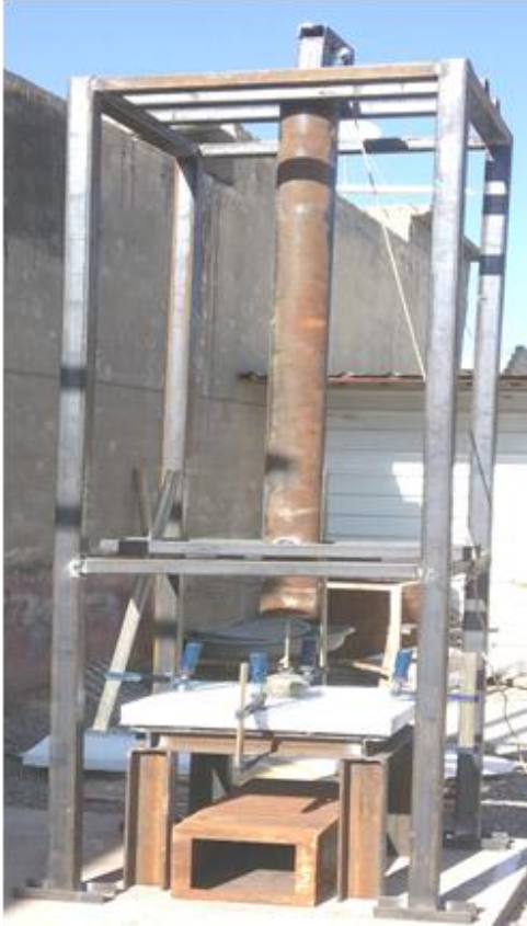
Plate (3): Frame test for impact loading
