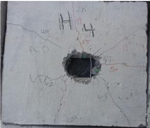
Plate (4): Failure of specimen under impact loading
